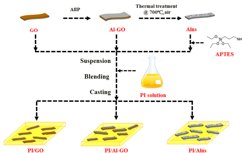
Figure 1. Schematic procedure to prepare fillers and PI nanocomposite films.
